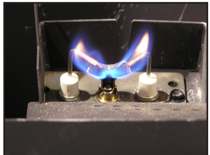
Figure 3.1 IPI Pilot Flame Patterns
